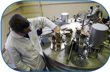
Upper flange of the SMES with the current leads and the cryocoolers
