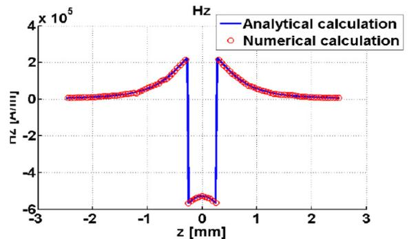
Figure 3 : Field created by a prismatic triangle magnet
