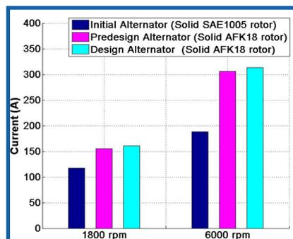
Improvement of output power with optimal FeCo core (FEM results)
