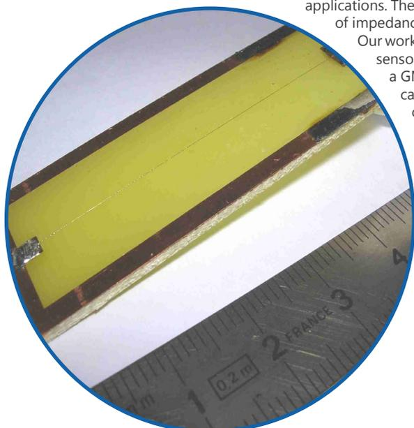
A typical GMI wire in the middle axis of the PCB
