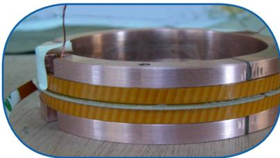
YBaCuO coil with outstanding performances: 1000 MA/m<sup>2</sup> under 18 T and hoop stress of 700 MPa
