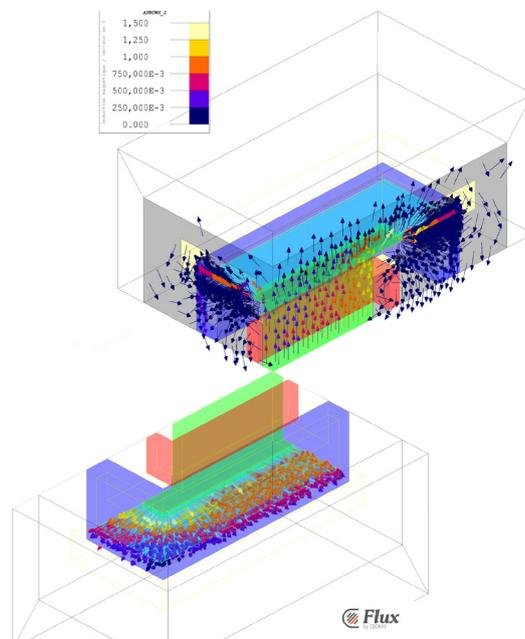
figure 2 : Flux 3D (Cedrat) simulation results (Magnetic Flux Density (Tesla) related to the specific device designed to apply magnetic field inside the furnace.
