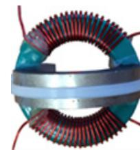
figure 3 : Prototype of integrated Common-Mode and Differential-Mode Choke with magnetic bypass over a tape wound core
