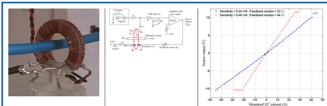
A GMI current sensor. The GMI wire has only one spire curled to a toroidal core. The measured current crosses the core; the windings around the core are used for the polarization and feedback.
