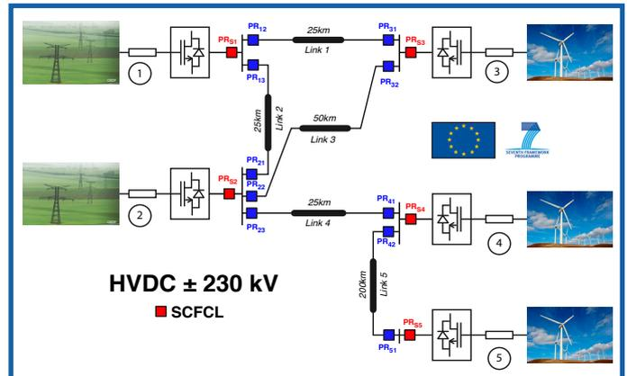
Figure 2 : Studied HVDC grid for wind farm connexions (Twenties EC project)
