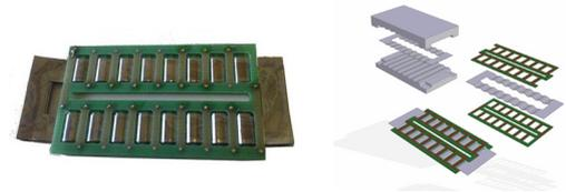
Figure 1 : View of the meander topology : stamping molds, meander magnetic core and up and bottom Print Circuit Board (Aperam Imphy Alloys / G2Elab) and PCB integrated prototype.
