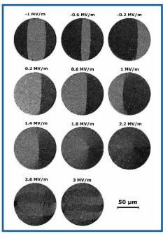
Direct magneto-optical Kerr observation of the rotation of the easy axis in 100 µm circular pods, for increasing values of the electric field applied to the demagnetized composite.
