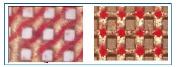
Diamagnetic latex beads (red) guided and matrixed above topographically patterned micro-magnet arrays (with Néel, Biopuces, LMGP)
