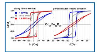
Normalized magnetic hysteresis cycles switched by applying opposite electrical fields, and measured along the fibres (easy axis) and perpendicular to the fibres (hard axis).
