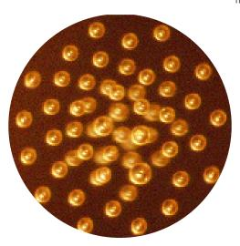
Top : Diamagnetic levitation of micro-droplets of water, mutually repulsed by their electrostatic charges.
