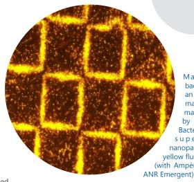
Magnetically-tagged bacteria trapped above an array of micromagnets. Flat 50x50 µm magnetic grid obtained by thermo-patterning. Bacteria having internalized s u p e r p a r a m a g n e t i c nanoparticles. Detection by yellow fluorescence. (with Ampère/ECL, Institut Néel -B Emergent)
