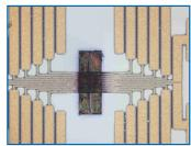
MEMS combining diamagnetic levitation and dielectrophoretic manipulation Left : principle. Right : integrated device (with LMGP, Néel, LTM LETI)
