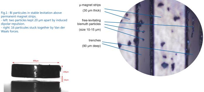
Fig.2 : double-dipole miniature magnet (phi 850 µm) in stable levitation 15 µm above polished graphite. The twin-magnet structure is visible in the reflection.
